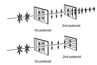
Figure 5.1 The action of polaroids
