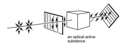
Figure 5.2 Rotation of the plane of plane-polarized light by an optically active substance
