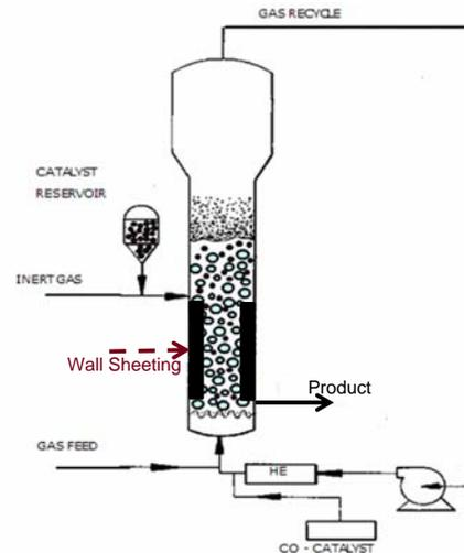
Figure: UNIPOL™ technology – Gas phase ethylene polymerization to produce polyethylene.
